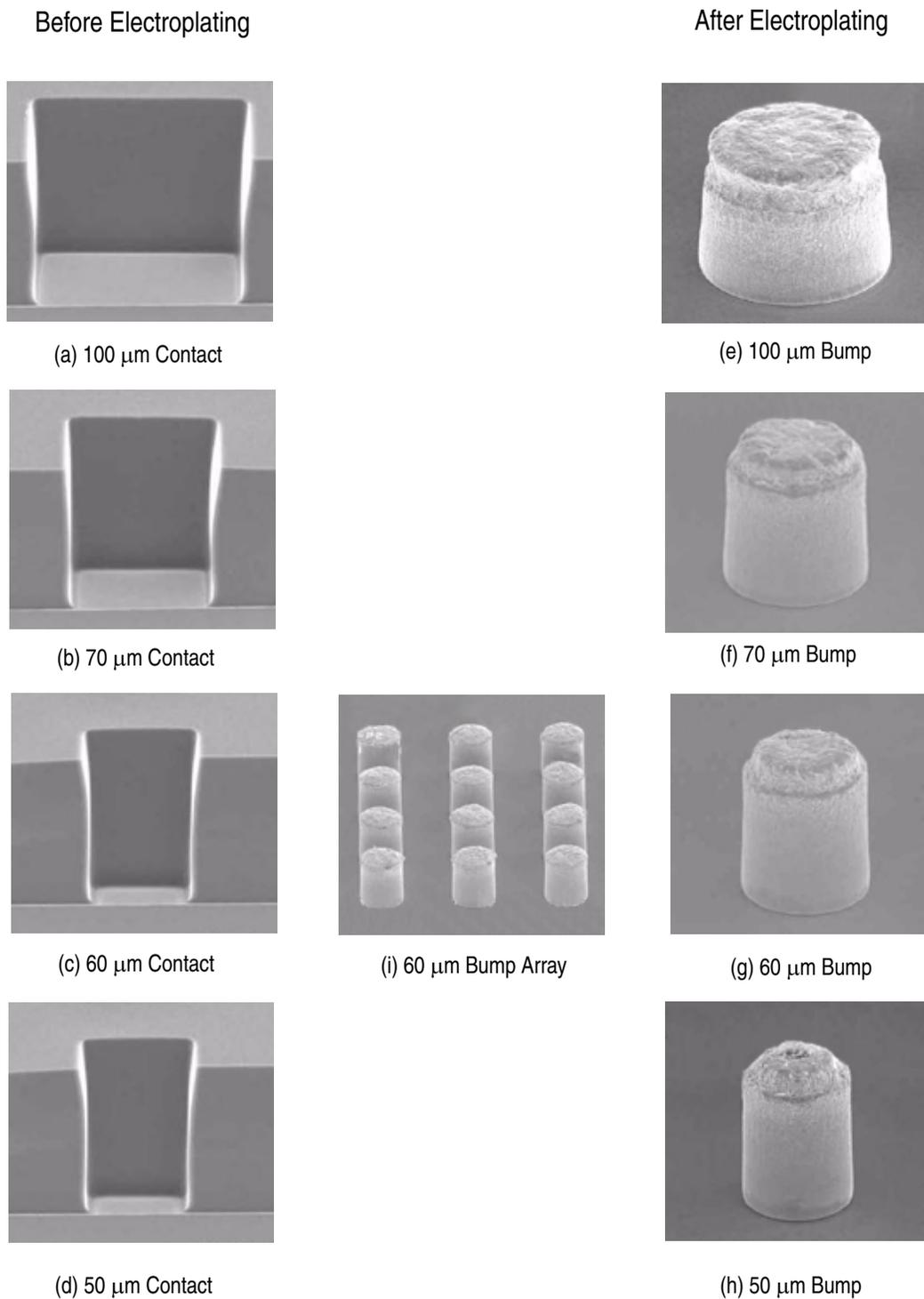
**Figure 7:** SEM Photographs illustrating the CD linearity of 100  $\mu\text{m}$  thick Shin-Etsu SIPR 7120 before and after electroplating. The photoresist images are a square contacts and the electroplated structures are round solder bumps. The exposure conditions are ghi-line exposure, -20  $\mu\text{m}$  focus, 5800  $\text{mJ}/\text{cm}^2$ .
