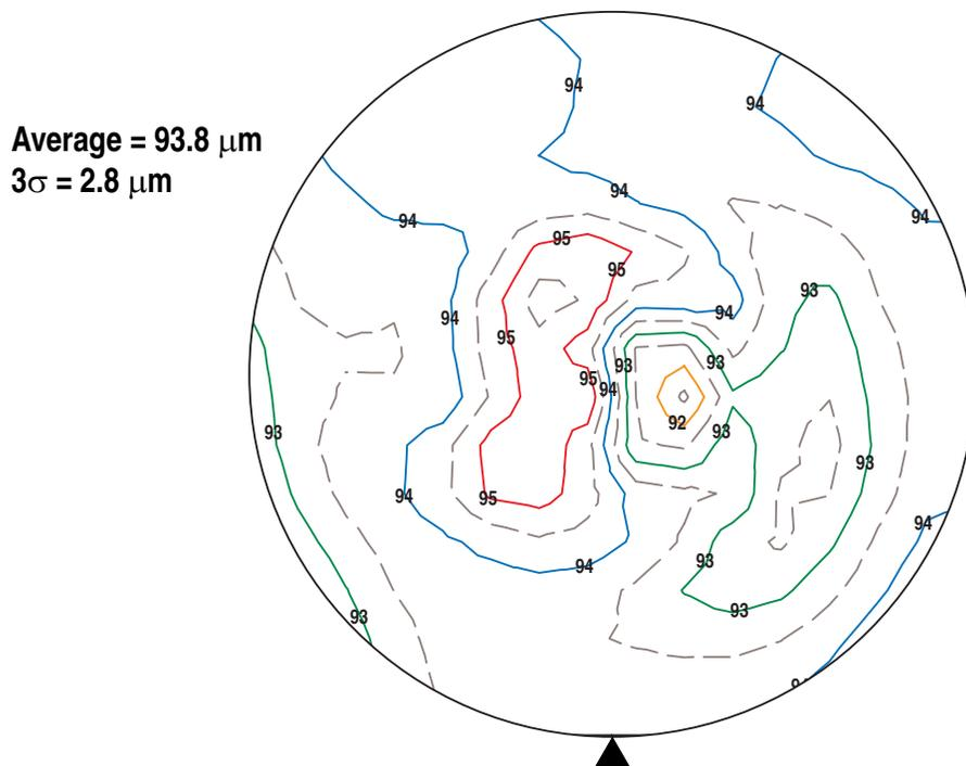
**Figure 4(b):** Enhanced coating uniformity for ShinEtsu SIPR 7120 on a 300 mm wafer after prebake. The solid contour lines are at 1.0  $\mu\text{m}$  intervals and the dashed contour lines are half way between. This coating process was not available in time to be used in this study.
