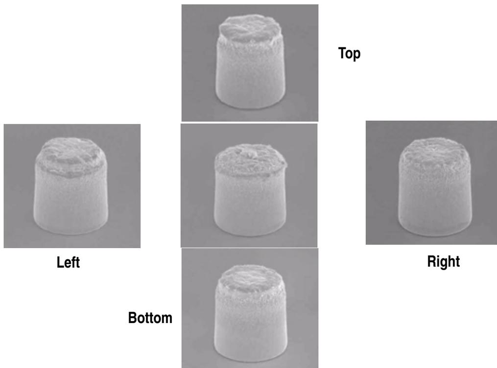
**Figure 6(b):** SEM Photographs of 70  $\mu\text{m}$  electroplated solder bumps showing CD uniformity on a 300 mm wafer.
