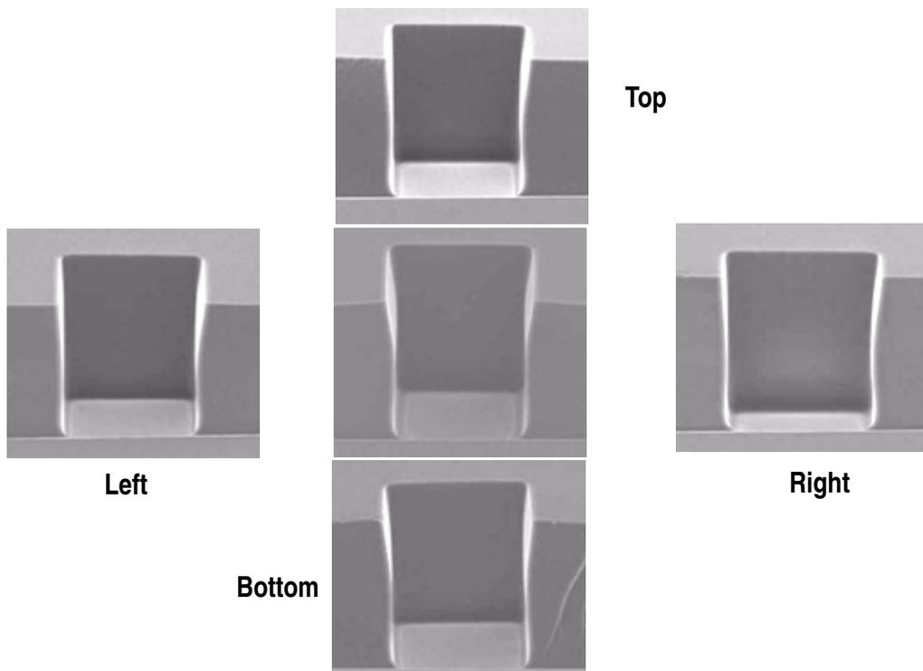
**Figure 5(b):** SEM Photographs of 70  $\mu\text{m}$  square contacts in SIPR 7120 showing CD uniformity on a 300 mm wafer.
