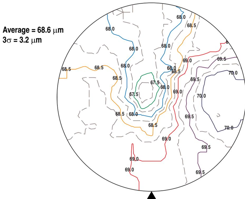
**Figure 5(a):** Photoresist CD uniformity of 70  $\mu\text{m}$  square contacts in ShinEtsu SIPR 7120 on a 300 mm wafer. The solid contour lines are at 0.5  $\mu\text{m}$  intervals and the dashed contour lines are half way between.
