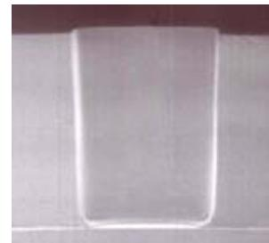
(g) Exposure = 5500 mJ/cm<sup>2</sup>, Focus= -20 μm
