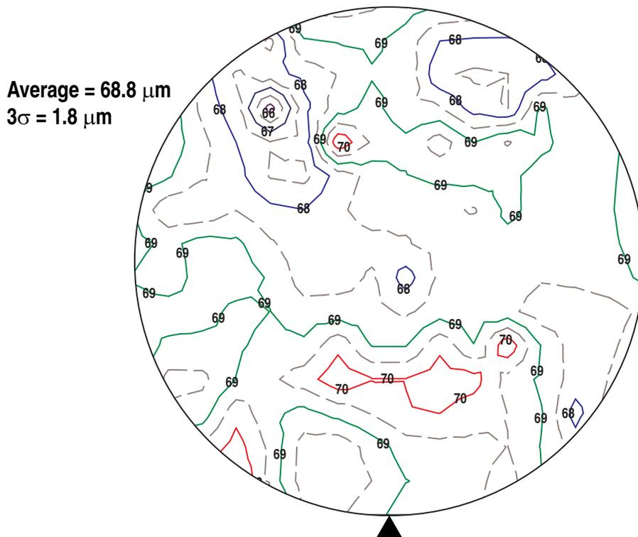
**Figure 6(a):** Electroplated CD uniformity of 70  $\mu\text{m}$  solder bumps on a 300 mm wafer. The solid contour lines are at 1.0  $\mu\text{m}$  intervals and the dashed contour lines are half way between.
