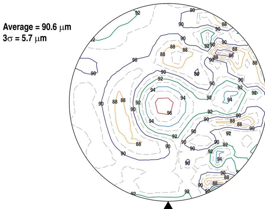
**Figure 4(a):** Coating uniformity for ShinEtsu SIPR 7120 on a 300 mm wafer after prebake. The solid contour lines are at 2.0  $\mu\text{m}$  intervals and the dashed contour lines are half way between. This is the coating process used in this study.
