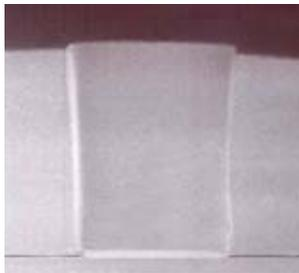
(c) Exposure = 5800 mJ/cm<sup>2</sup>, Focus= -20 μm
